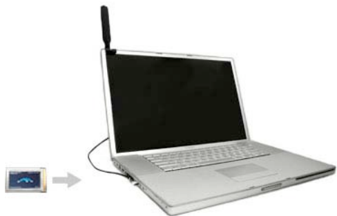
Laptop equipped with Ubiquiti SR4C + external antenna
