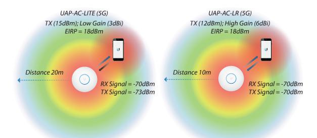
The antenna gain diagrams represent a three-dimensional area over which wireless signals propagate. Indoor as well as outdoor UniFi access points feature 'omnidirectional' antennas that produce a radiation pattern similar to a 'donut' shape.
