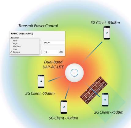
The purpose of any access point is to provide wireless coverage to clients over a given area known as a cell. As a WLAN station moves away from the AP, its receive signal gradually weakens. This also occurs as obstacles prevent direct line-of-sight between AP and station. As signals decrease, wireless performance drops before eventually, the station becomes disconnected from the AP. This is due to the Free Space Path Loss (FSPL) relationship as mentioned previously.
