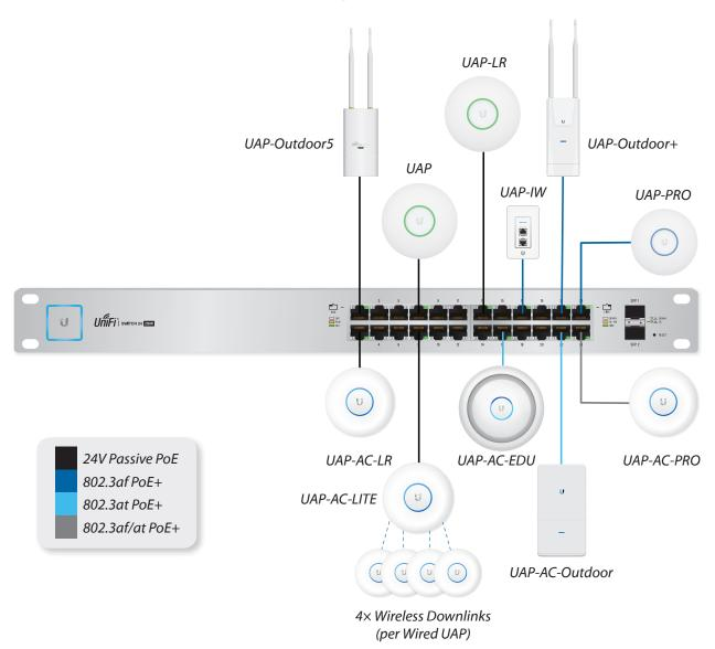
Despite its name, "wireless" networks still rely on cables and wires to connect access points to switches and routers. It's imperative that Ethernet connections function properly in full duplex and at advertised data rates (100/1000 Mbps), otherwise bottlenecks will occur. These problems can occur when line and EMI interference is present. Whenever possible, use outdoor-rated, shielded-twisted pair (STP) Ethernet cables like TOUGHCable to protect against harsh weather and RF environments.
