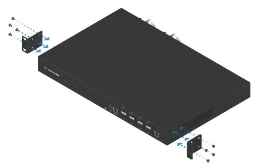
Attaching Rack-Mount Brackets to the EdgeRouter Infinity
