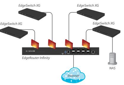
The EdgeRouter Infinity connects to multiple 10G EdgeSwitch® XG units.
